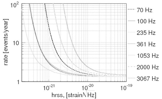
**Figure 2.** Upper limits on the rate of gravitational wave bursts, determined using the LIGO and Virgo data. The different curves represent signals with different characteristic frequencies; the vertical position of each curve shows what rate should have given us at least one detectable burst with 90% probability, for different assumptions about the strength of the burst (horizontal axis). Since *no* signal was detected, higher rates are ruled out with good confidence.
