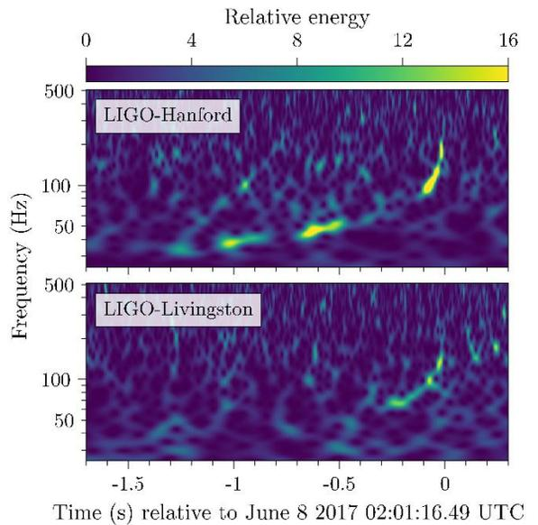
**Figure 2.** Energy in LIGO data as a function of time in seconds along the X axis and frequency in Hertz along the Y axis. The colors indicate the amount of energy at any given time/frequency, going from blue (low) to yellow (high). The curve from the lower left to the upper right, clearly visible in the Hanford data and hinted at in the Livingston data, is the gravitational wave signal from the black hole inspiral. (Adapted from Figure 1 in the [paper](#)).
