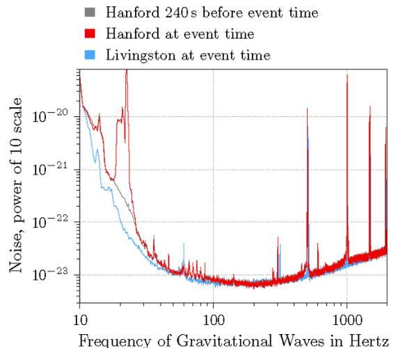
**Figure 1.** Sensitivity of the LIGO detectors at both Hanford and Livingston, shown as noise on the Y axis and gravitational wave frequency on the X axis. The Hanford graph shows noise 4 minutes before the event (grey) which was before the commissioning activity started, and noise during the event (red). Note the much larger noise between about 20 Hertz and 30 Hertz at Hanford during the event. The noise at the Livingston detector is shown in blue. (Adapted from Figure 4 in the [paper](#)).
