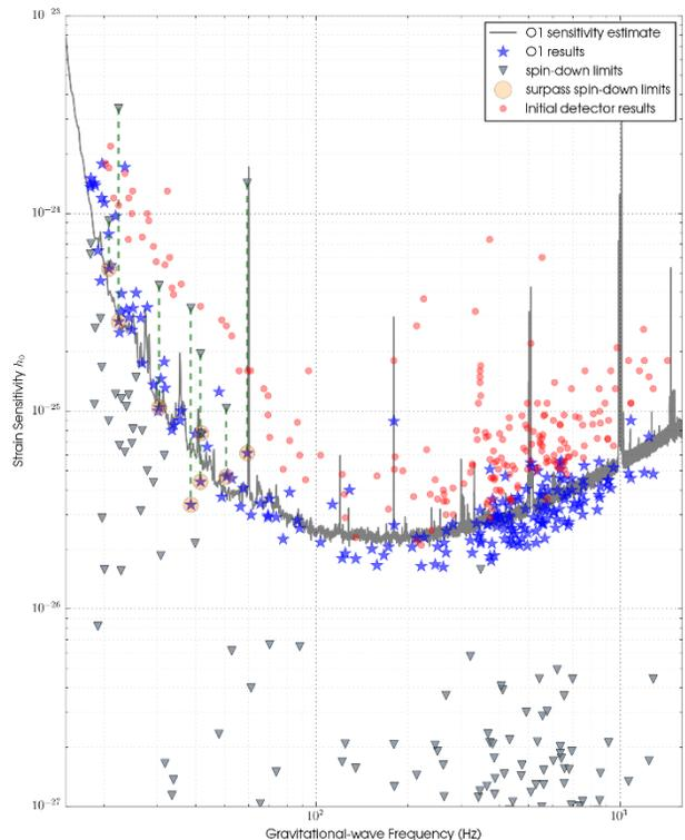
The stars in this plot show the [upper limits](#) on the gravitational wave [strain amplitude](#) for 200 pulsars using data from the first Advanced LIGO observing run. The triangles show the [spin-down limits](#) for these stars. The pulsars for which our observations have surpassed the spin-down limits are highlighted with circles. The curve gives an estimate of the expected sensitivity of the run.
