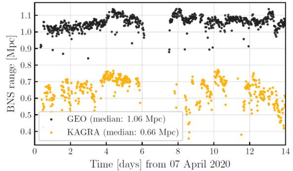
**Figure 2:** (The right panel of Fig. 1 from our publication) The BNS observable ranges for KAGRA (yellow) and GEO (black) during the joint observing run. The evolution of the ranges during the observing run is shown. The gap around day 6 and 7 was caused when both detectors were affected by bad weather and were unable to lock. The median range values are 0.66 megaparsecs for KAGRA and 1.06 megaparsecs for GEO.
