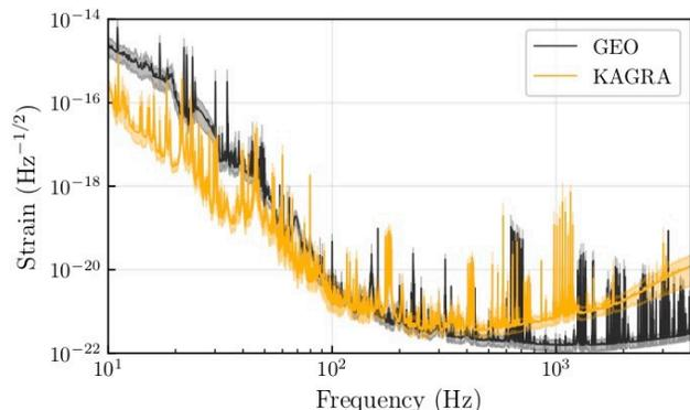
**Figure 1:** (The left panel of Fig. 1 from our publication) Plot showing the typical sensitivity of KAGRA (yellow) and GEO (black) during the joint observing period. The vertical axis gives the average **strain noise** in the detectors, which is a measure of how much the mirrors typically move as a function of frequency (horizontal axis). The solid curves show the mean sensitivity for each frequency bin and the shaded regions show the 5th and 95th percentile over the period.
